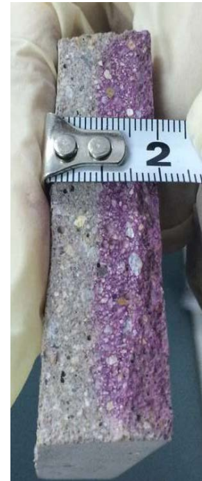
Figure 4: Carbonation depth of 10 mm (gray color) after 6 months in outdoor conditions in Shenyang, China. Figure from Xi et al. (supplement, tab “SI data 15”)
