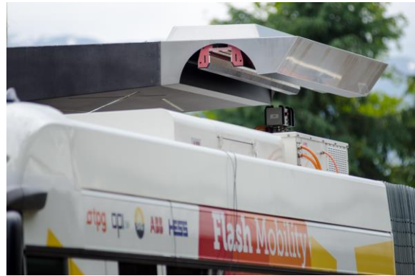
Figure 4. Electric Bus Charging in Geneva (Source: ABB)
