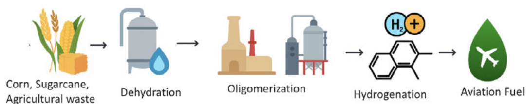
FIGURE 2.2.2: Process flow and system boundary for ATJ.
