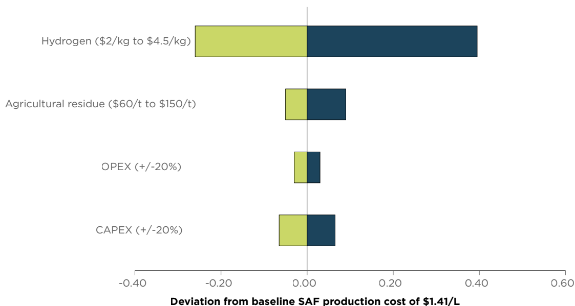
FIGURE A.2.6 Impact of varying key assumptions on the levelized cost of PBtL SAF production.
