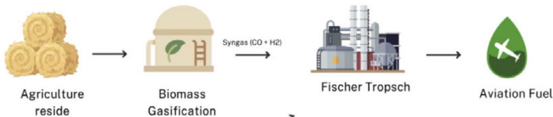
FIGURE 2.2.3: Process flow and system boundary for BtL.
