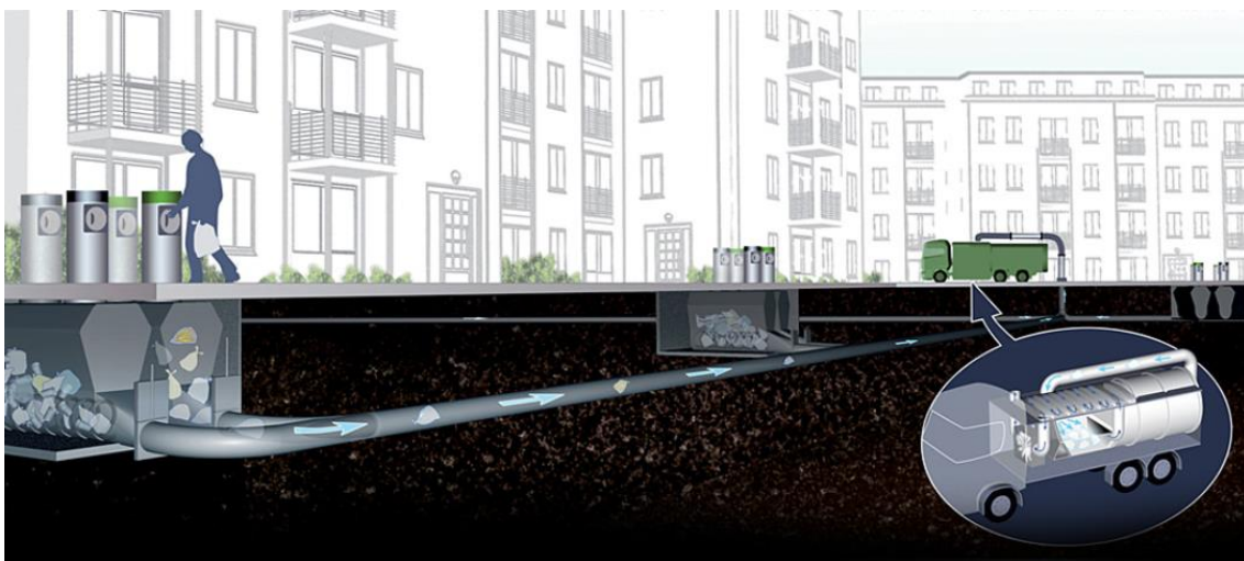
Figure 63. Mobile vacuum system in Hammarby Sjöstad. Source: City of Stockholm
